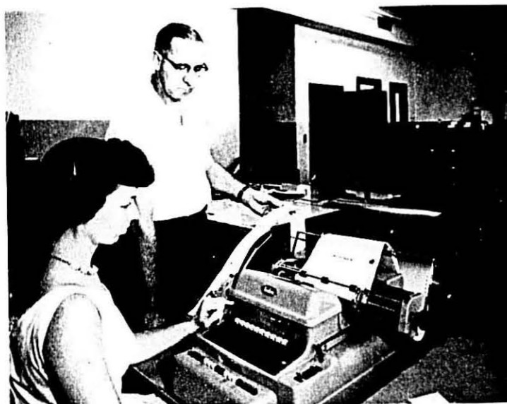
Delmonico Office Manager Arthur O'Toole watches as edge-punched card feeds item information for automatic writing by Computyper.
